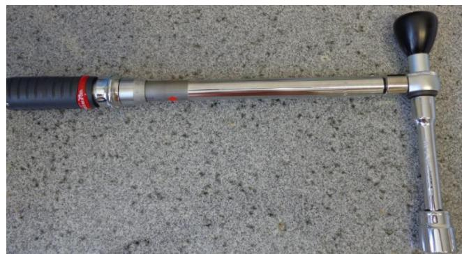
*Figure 6. Torque wrench to close the autoclave*
