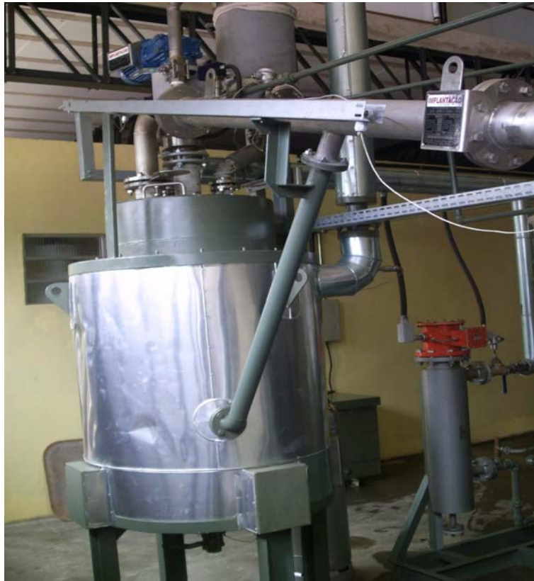
Figure 3. 2 - Stirred Sludge Bed Reactor (R-01).
